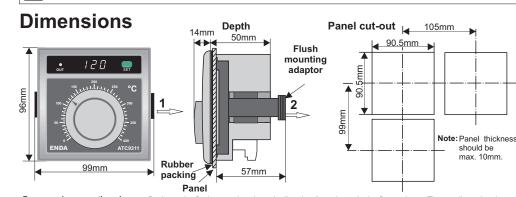
For removing mounting clamps : Push out the flush-mounting clamp in direction 1 as shown in the figure above. Then, pull out the clamp in direction 2. If there is no 60mm free space at back side of the device, it would be difficult to remove it from the panel.
