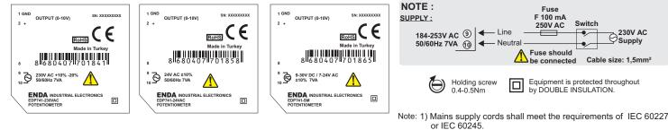
2) In accordance with the safety regulations, the power supply switch shall bring the identification of the relevant instrument and it should be easily accessible by the operator.
