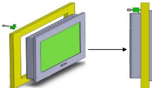
Put the unit through the panel cut out. Slide the clamps into the 4 holes provided around the case. Tighten the clamping screws in an even pattern until the unit is secured in the panel.
